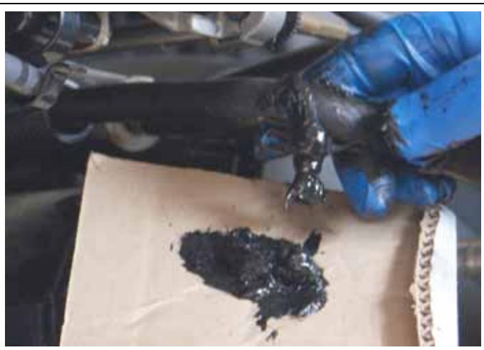
Fuel hose dissolved from contaminated fuel
