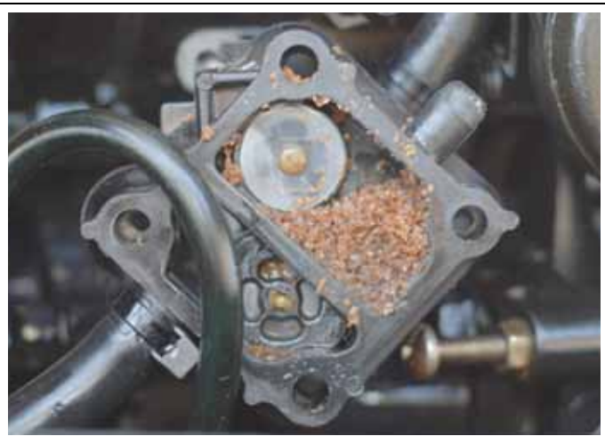
Fuel pump – gelled deposit
