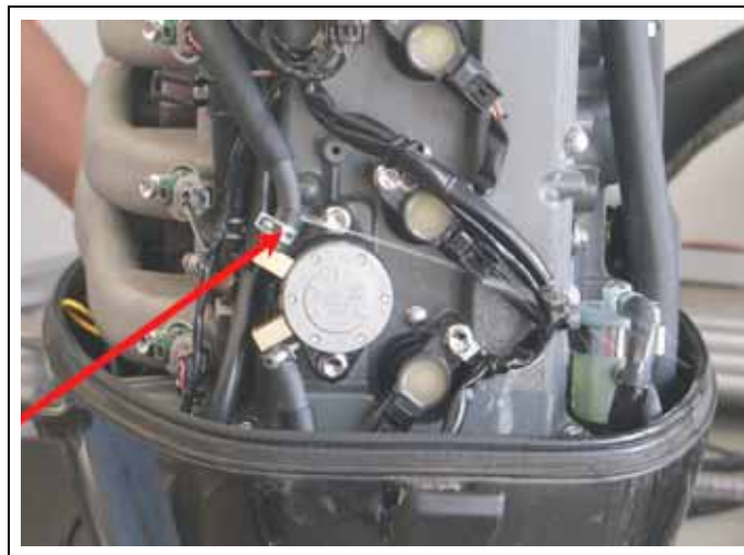
Fuel leak caused by hose damaged from contaminated fuel
