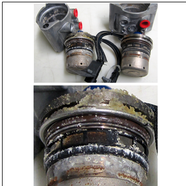
Fuel Contaminated Injectors and Mounting Cups
