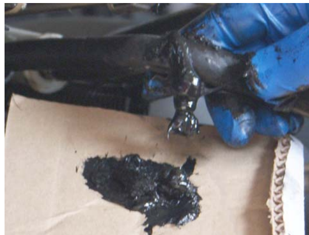
Blockage in the fuel system
