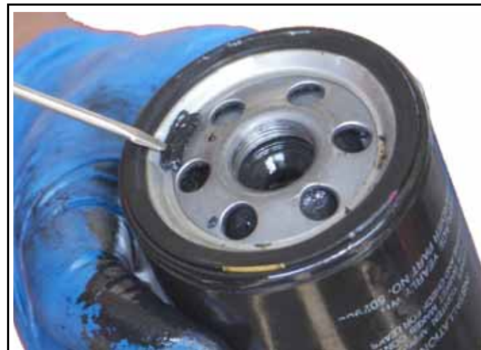
Deteriorated hose pieces trapped by fuel filter
