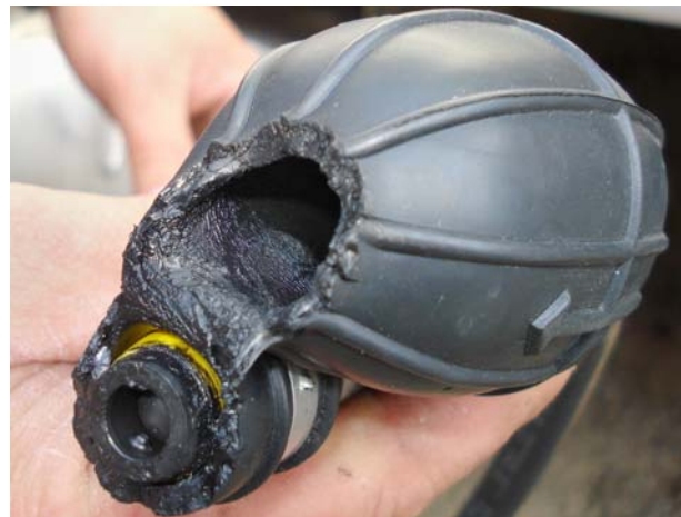
Deteriorated fuel hose and primer bulb
