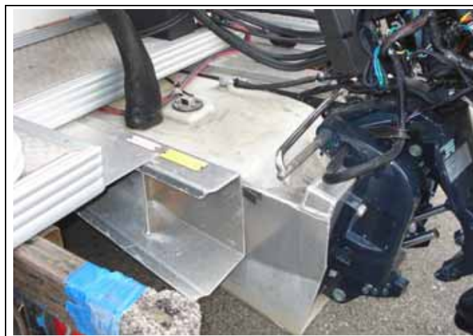
Monitor fuel tanks in unique applications carefully for water in fuel
