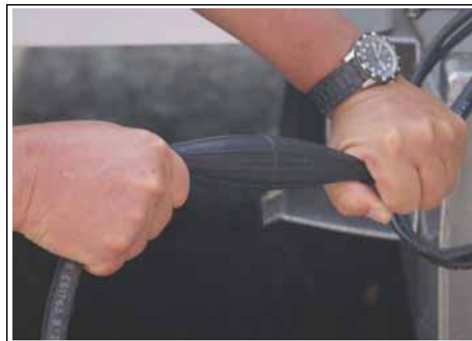
Damaged fuel primer bulb
